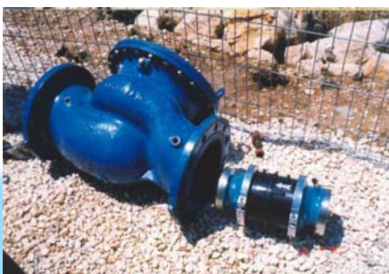
Photograph showing the size of a C-valves M-1 body (right) used to replace an existing PRV.
