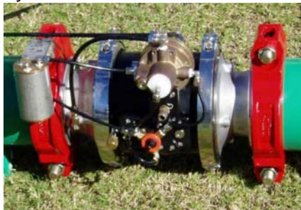
Photograph showing the 150mm C-Valves PFR with modular baseplate, 3 way pilot and filter before installation within Wide Bay Water's Hervey Bay water distribution system
